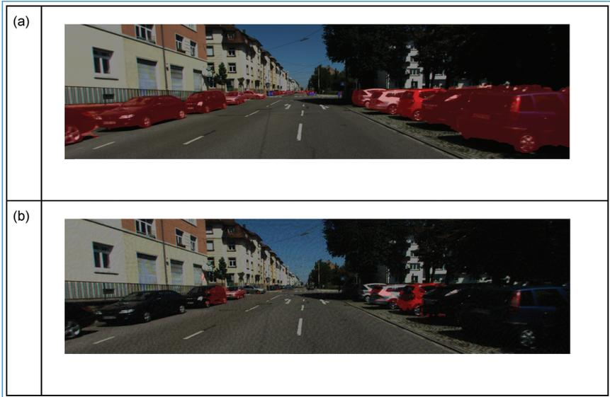
**Figure 18.** Image (a) is the output of the segmentation model to the non-attacked image while in the image (b) is the output of the segmentation model to the attacked image. The red mask indicates the detected vehicles.
