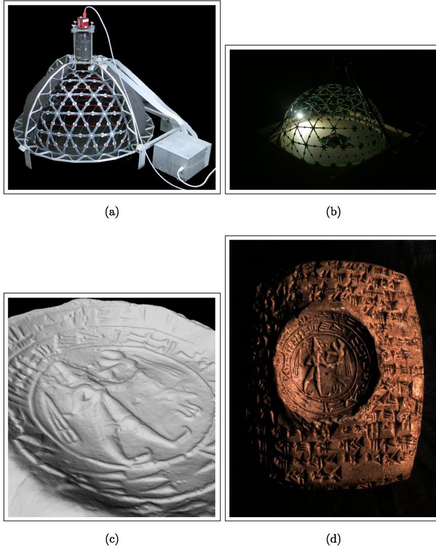
Fig. 1.9 (a) Mini-dome with different LED light sources, (b) scene with one of the LEDs activated, (c) 3D reconstruction of a cuneiform tablet, without texture, and (d) the same tablet with texture.
