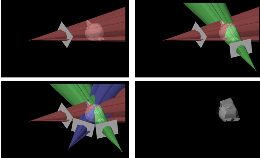
Fig. 1.11 The first three images show different backprojections from the silhouette of a teapot in three views. The intersection of these backprojections form the visual hull of the object, shown in the bottom right image. The more views are taken, the closer the visual hull approaches the true shape, but cavities not visible in the silhouettes are not retrieved.
