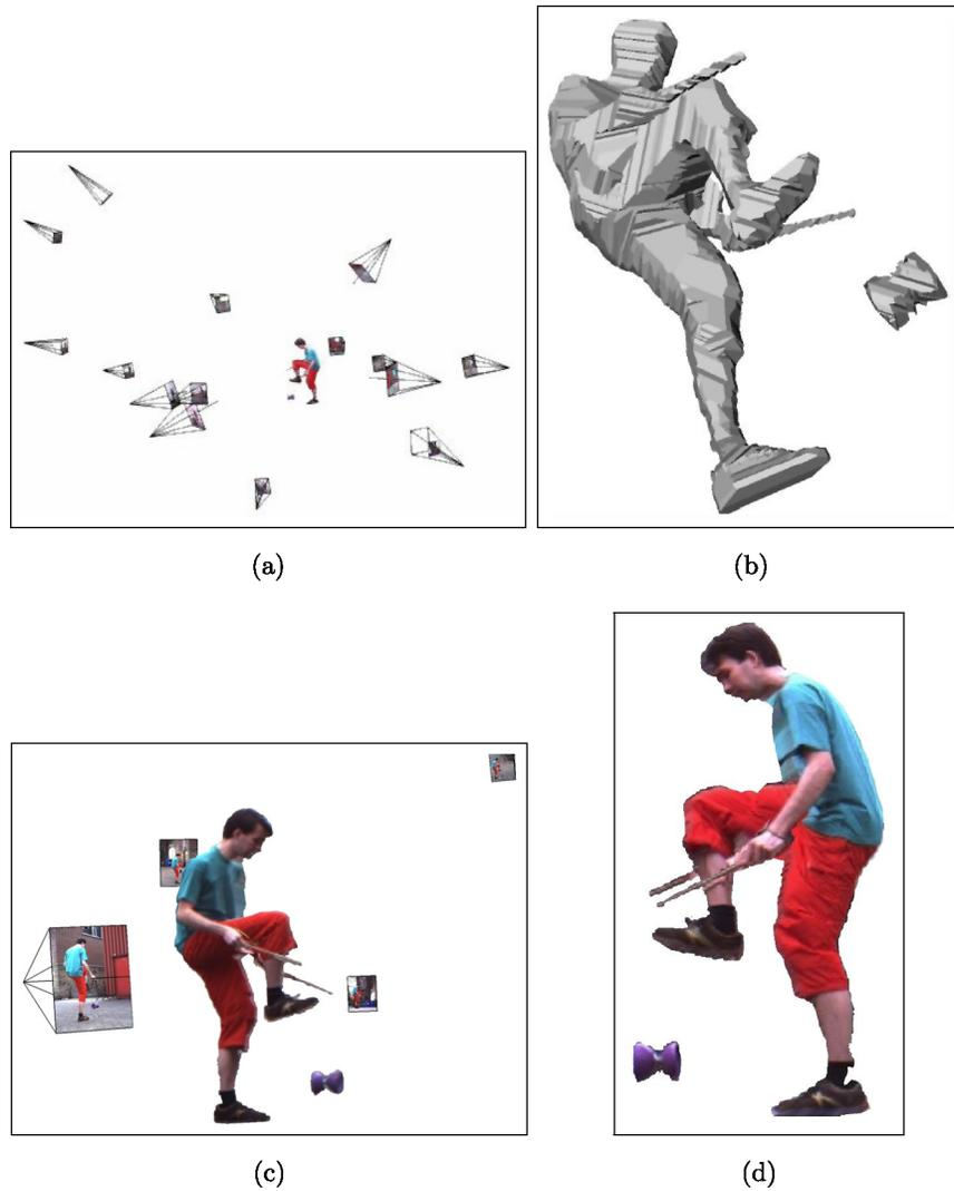
Fig. 1.12 (a) Fifteen cameras setup in an outdoor environment around a person,(b) a more detailed view on the visual hull at a specific moment of the action,(c) a detailed view on the visual hull textured by backprojecting the image colors, and (d) another view of the visual hull with backprojected colors. Note how part of the sock area has been erroneously carved away.
