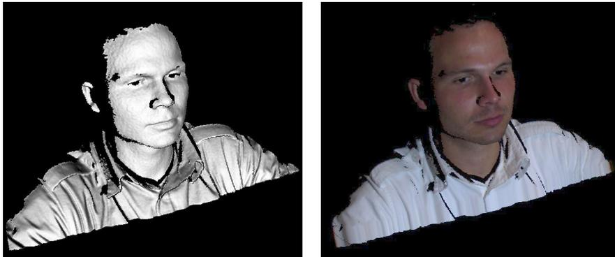
Fig. 1.6 3D results obtained with a phase-shift system. *Left:* 3D reconstruction without texture. *Right:* The same 3D reconstruction with texture, obtained by summing the three images acquired with the phase-shifted sine projections.
