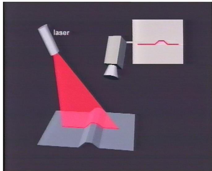
Fig. 1.4 If the active triangulation configuration is altered by turning the laser spot into a line (e.g., by the use of a cylindrical lens), then scanning can be restricted to a one-directional motion, transversal to the line.
