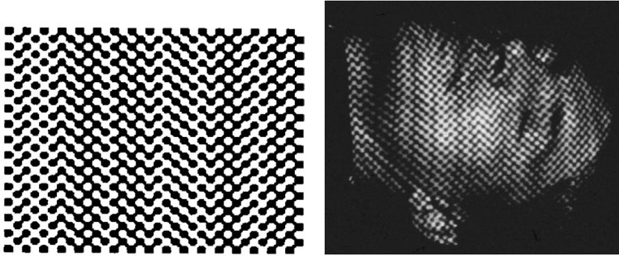
Fig. 1.7 Example of one-shot active range technique. *Left*: The projection pattern allowing disambiguation of its different vertical columns. *Right*: The pattern is projected on a face.
