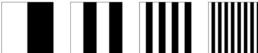
Fig. 1.5 A series of masks that can be projected for active stereo applications. Subsequent masks contain ever finer stripes. Each of the masks is projected and for a point in the scene the sequence of black/white values is recorded. The subsequent bits obtained that way characterize the horizontal position of the points, i.e., the plane of intersection (see text). The resolution that is required (related to the width of the thinnest stripes) imposes the number of such masks that has to be used.
