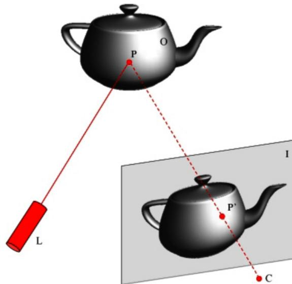
Fig. 1.3 The triangulation principle used already with stereo, can also be used in an active configuration. The laser  $L$  projects a ray of light onto the object  $O$ . The intersection point  $P$  with the object is viewed by a camera and forms the spot  $P'$  on its image plane  $I$ . This information suffices for the computation of the three-dimensional coordinates of  $P$ , assuming that the laser-camera configuration is known.
