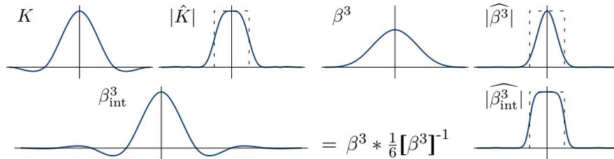
**Figure 1.4:** The traditional Keys cubic (Catmull-Rom spline)  $K$  has support 4 and a reasonably sharp frequency response  $|\hat{K}|$ . The cardinal cubic B-Spline  $\beta_{\text{int}}^3$  is a generalized kernel formed from the basic cubic B-spline  $\beta^3$  and a digital filter. The digital filter acts to widen support to infinity (though with exponential decay) and to significantly sharpen the frequency response.
