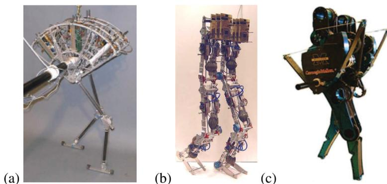
**Figure 1.7:** Compliant bipeds (a) Spring Flamingo with linear SEAs and (b) Lucy with variable compliance pneumatic artificial muscles and (c) MABEL actuated using a nonlinear leaf spring to provide compliance along the virtual leg.
