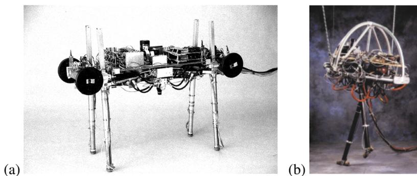
**Figure 1.5:** (a) Raibert's quadruped and (b) 3D biped.
