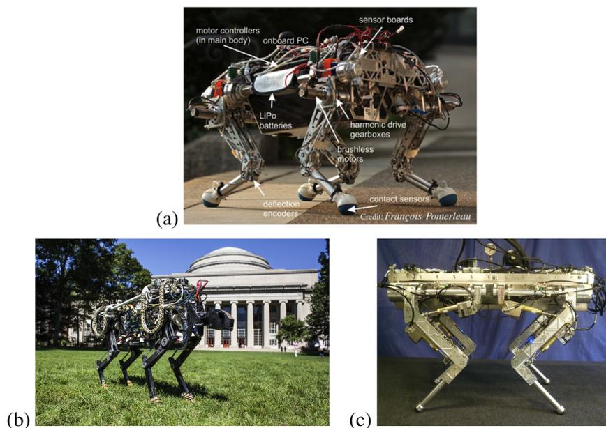
**Figure 1.10:** Modern Quadrupeds (a) StarlETH (b) MIT Cheetah 2 and (c) HyQ.
