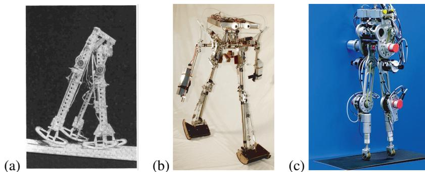
**Figure 1.6:** Bipeds on the spectrum of passive design. (a) Tad McGeer’s passive 2D walker (b) A 3D, minimally actuated walker designed by Collins and Ruina and (c) RABBIT, an underactuated point-foot biped.
