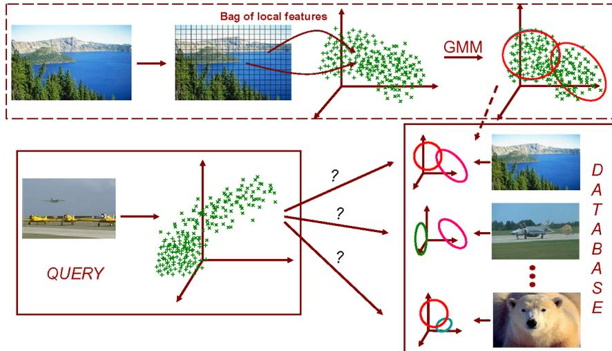
Fig. 1.1 MPE retrieval architecture. Images are decomposed into bags of local features, and characterized by their distributions on feature space. Database images are ranked by posterior probability of having generated the query features.
