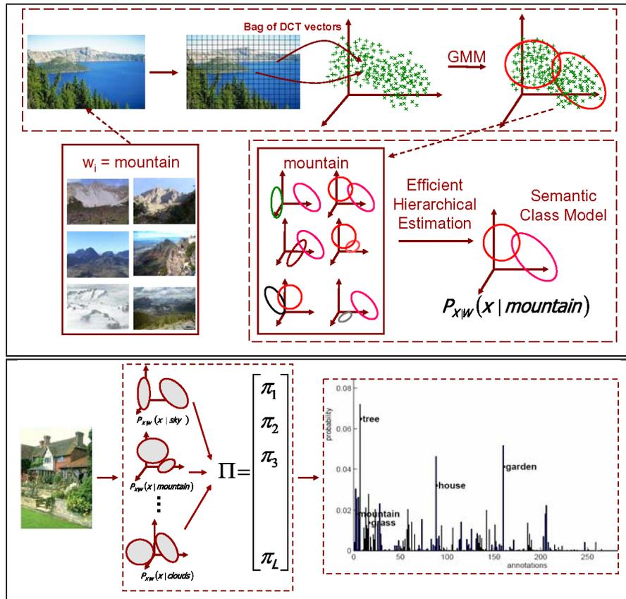
Fig. 1.4 Semantic MPE labeling. Top: images are grouped by semantic concept, and a probabilistic model learned for each concept. Bottom: each image is represented by a vector of posterior concept probabilities.
