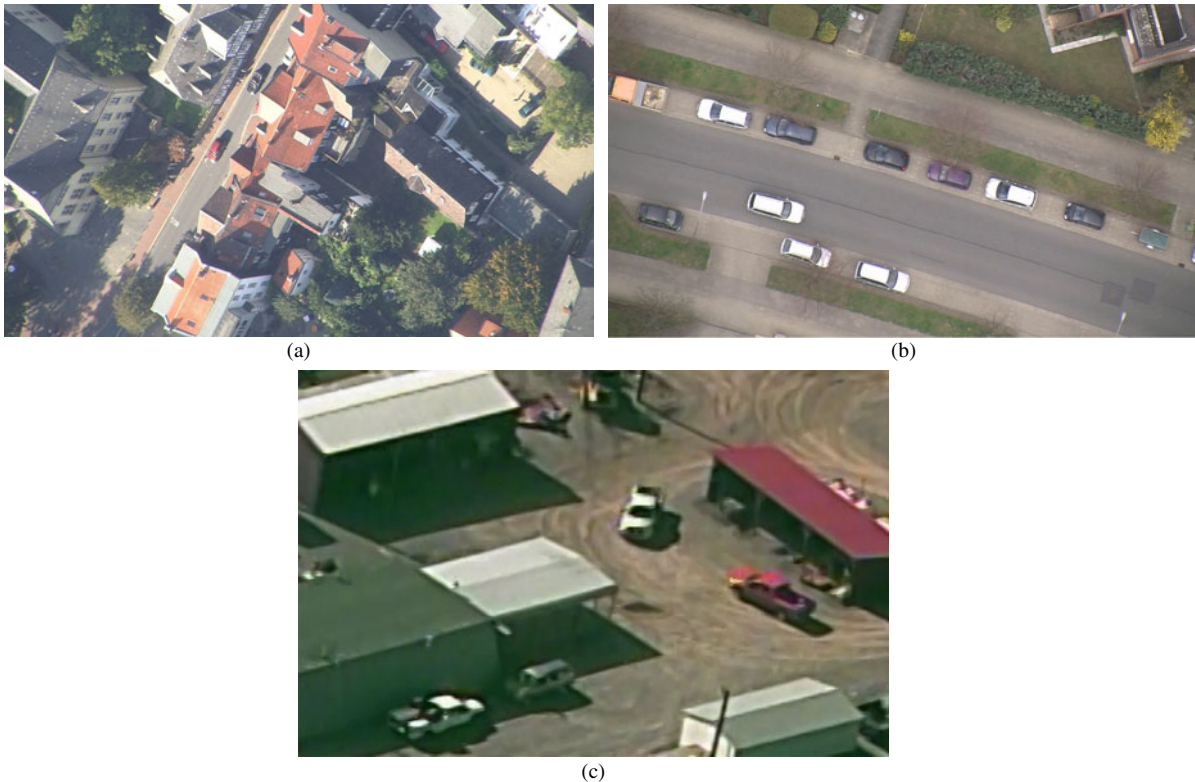
Fig. 7. Example frames of the test set used to evaluate the MO detection and ROI coding framework. ( Test Set 1 ). (a) MOs (black and red car with shadows) in the 750 m sequence, HDTV resolution, ground resolution: 21 pel/m [34, 39]. (b) MO (white car in the middle) in the 350 m sequence, HDTV resolution, ground resolution: 43 pel/m [34, 39]. (c) MOs (white and red car in the middle) in the VIRAT test data set, original resolution: 720 \times 480 , interlaced [37, 38].
