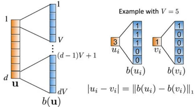
Fig. 4. “Unary” expansion of an integer vector to preserve  $\ell_1$  distances. Each element of the original vector is expanded to  $V$  bits, such that if the coefficient value is  $u_i$ , the first  $u_i$  bits are set to 1 and the next  $V - u_i$  bits are set to zero. The  $\ell_2$  distance between expanded vectors equals the  $\ell_1$  distance between the original vectors. This requires that  $u_i$  is bounded by  $V$ . Thus, a  $d$ -dimensional vector is expanded to  $dV$  dimensions.
