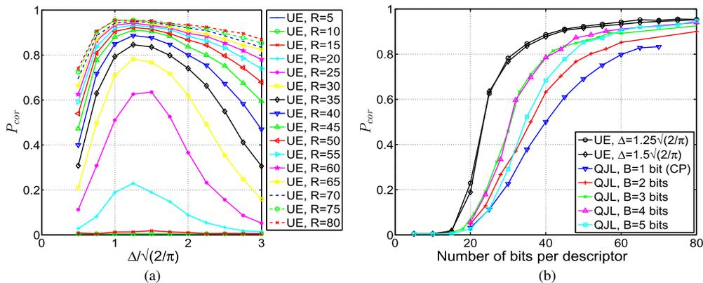
Fig. 7. (a) Universal embedding performance at different bit rates, as a function of  $\Delta$  (b) Performance of properly tuned universal embeddings (UE) as a function of the rate, compared with the conventionally quantized JL embeddings (QJL) also shown in Fig. 6(b).
