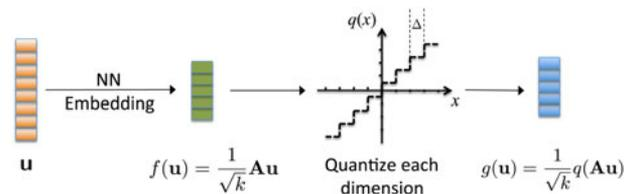
Fig. 2. (a) A quantized embedding is derived by first obtaining a JL embedding by multiplying the vectors in the canonical feature space by a random matrix, followed by scalar quantization of each element in the vector of randomized measurements.
