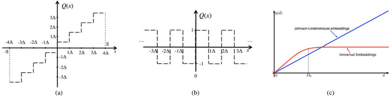
Fig. 5. (a) Conventional 3-bit (eight levels) scalar quantizer with saturation level  $S = 4\Delta$ . (b) Universal scalar quantizer. (c) The embedding map  $g(d)$  for JL-based embeddings (blue) and for universal embeddings (red).
