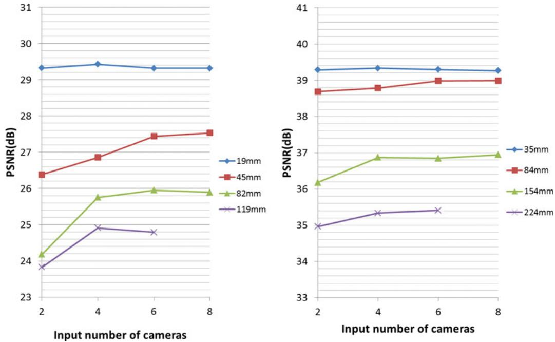
Fig. 10. PSNR using different number of cameras (left: “Bee”, right: “Shark”). The values in the legend shows the baseline distance between each reference viewpoint images.
