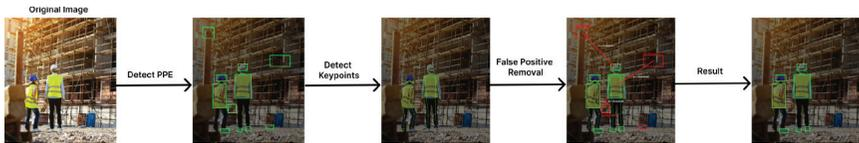
Figure 6: False Positive Removal Mechanism.
