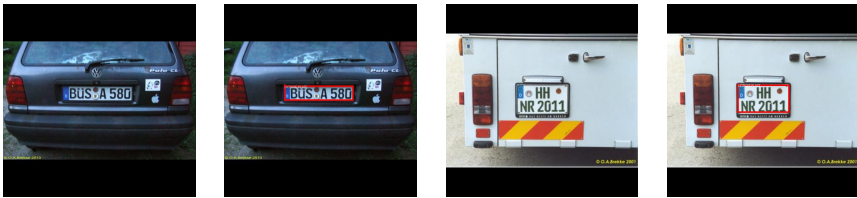
Figure 6: License plate detection results using the LPD model. The red bounding boxes indicate the localized license plate regions. The first and third images (from the left) show the input images, while the second and fourth images display the corresponding detection outputs.
